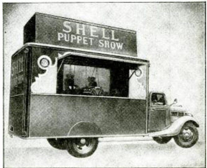
Wild motorists, known to cops as "cowboys", to Shell Oil Co. as "screw-drivers," receive visual message from puppet show in truck above, audible message from Lafayette model 269-T mobile amplifier installed in truck. Power from 1,500-W. generator provides system's power, floodlighting, stage-lighting, etc. Job has record player, mixer, fader, etc. Output 20 W. to two 10-in. speakers.
