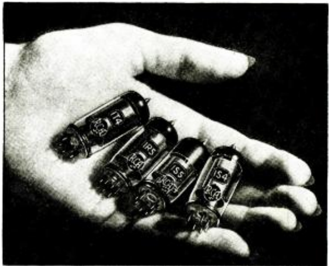
At last! Miniature tubes not designed for any special purpose! They can be used wherever ordinary-size radio tubes of similar characteristics are employed. The series includes R.F., A.F. and power types.
